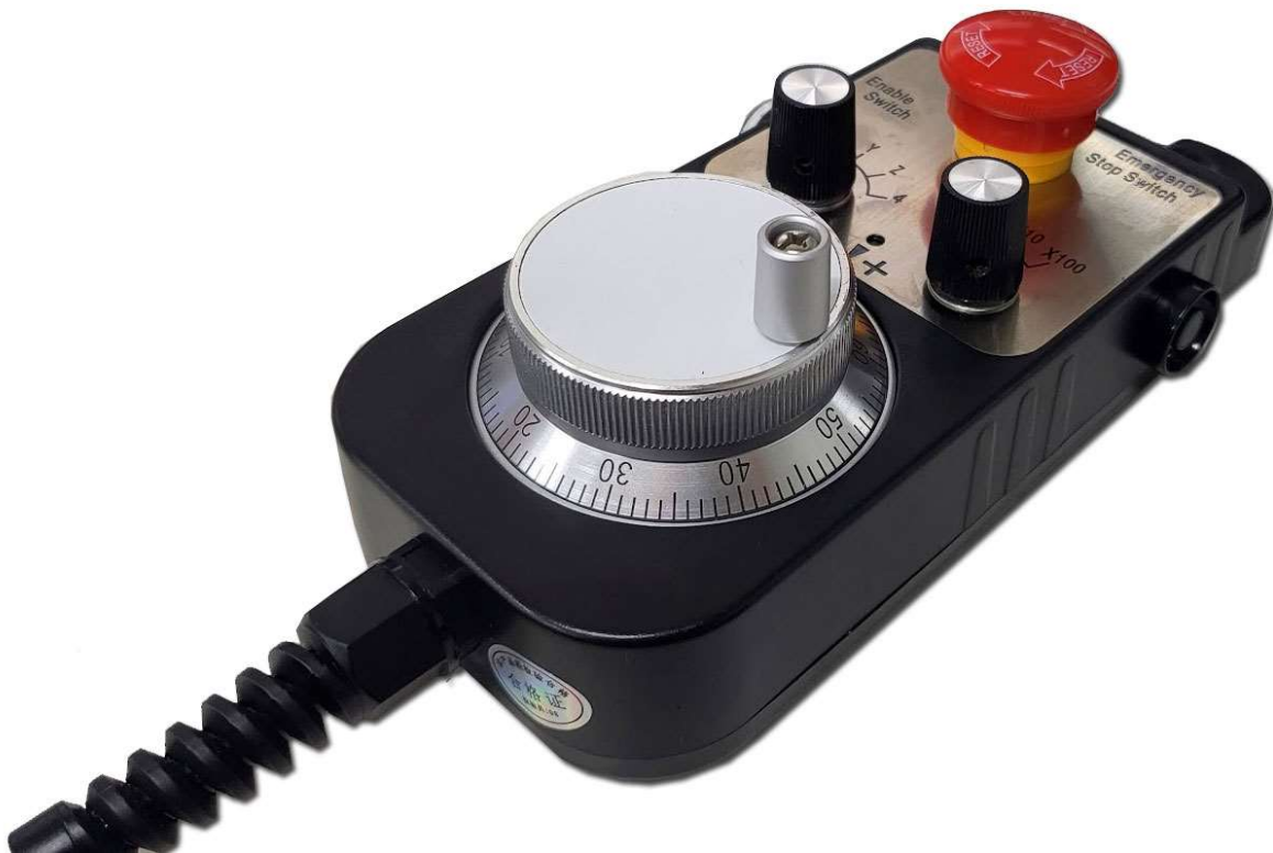
Figure 3-6: Control panel and pendant examples
